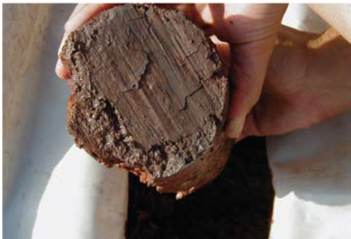
Figure 12. Slip lines observed on the slip surface of the Corinth core.
