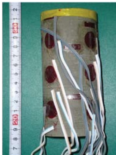
Figure 4. Anelastic strain recovery measurement of absolute stress on a core sample.
